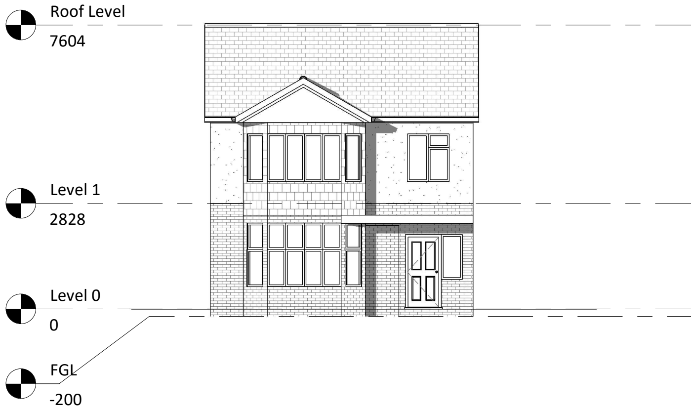
Existing Front Elevation
