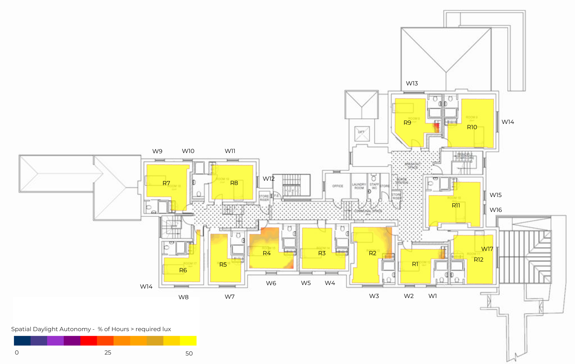
Figure 6: Spatial Daylight Autonomy (SDA) results for habitable rooms on first floor (with window and room references).
