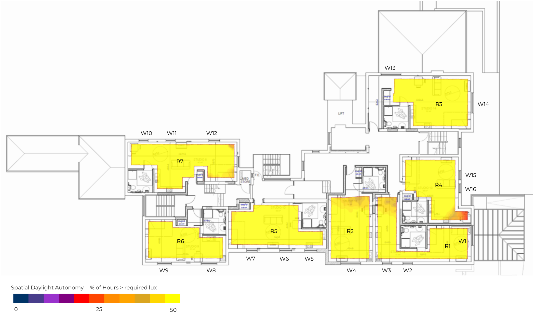
Figure 6: Spatial Daylight Autonomy (SDA) results for habitable rooms on first floor (with window and room references).
