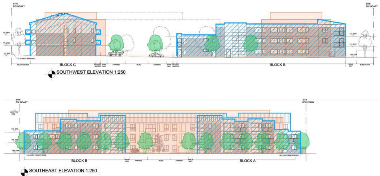
Figure 15: Detailed elevation of the proposal, with the outline of the approved scheme in a blue dotted line demonstrating that the marginal increase in height and bulk of the proposal is minimal
