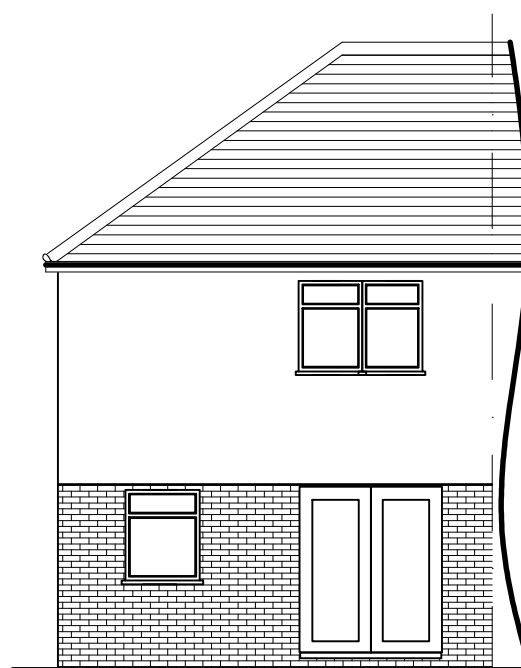
EXISTING REAR ELEVATION OF 27 1:100
