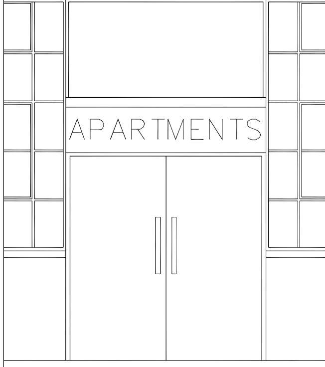
TYPICAL ENTRANCE DOOR ELEVATION Scale 1:20 @ A1
