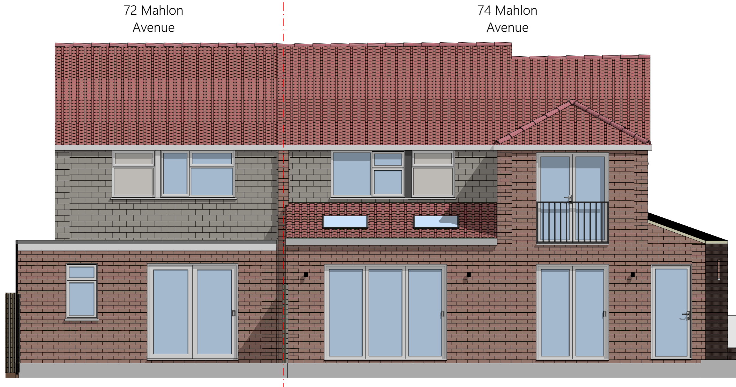
Proposed Rear Elevation Scale: 1:50
