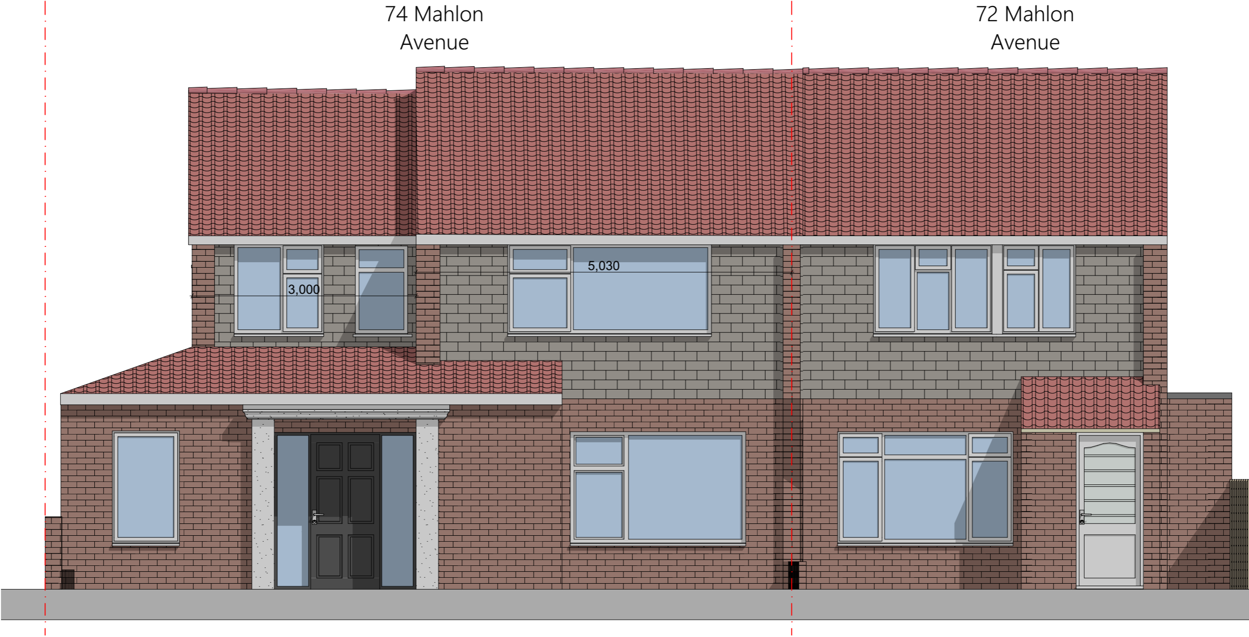
Proposed Front Elevation Scale: 1:50
