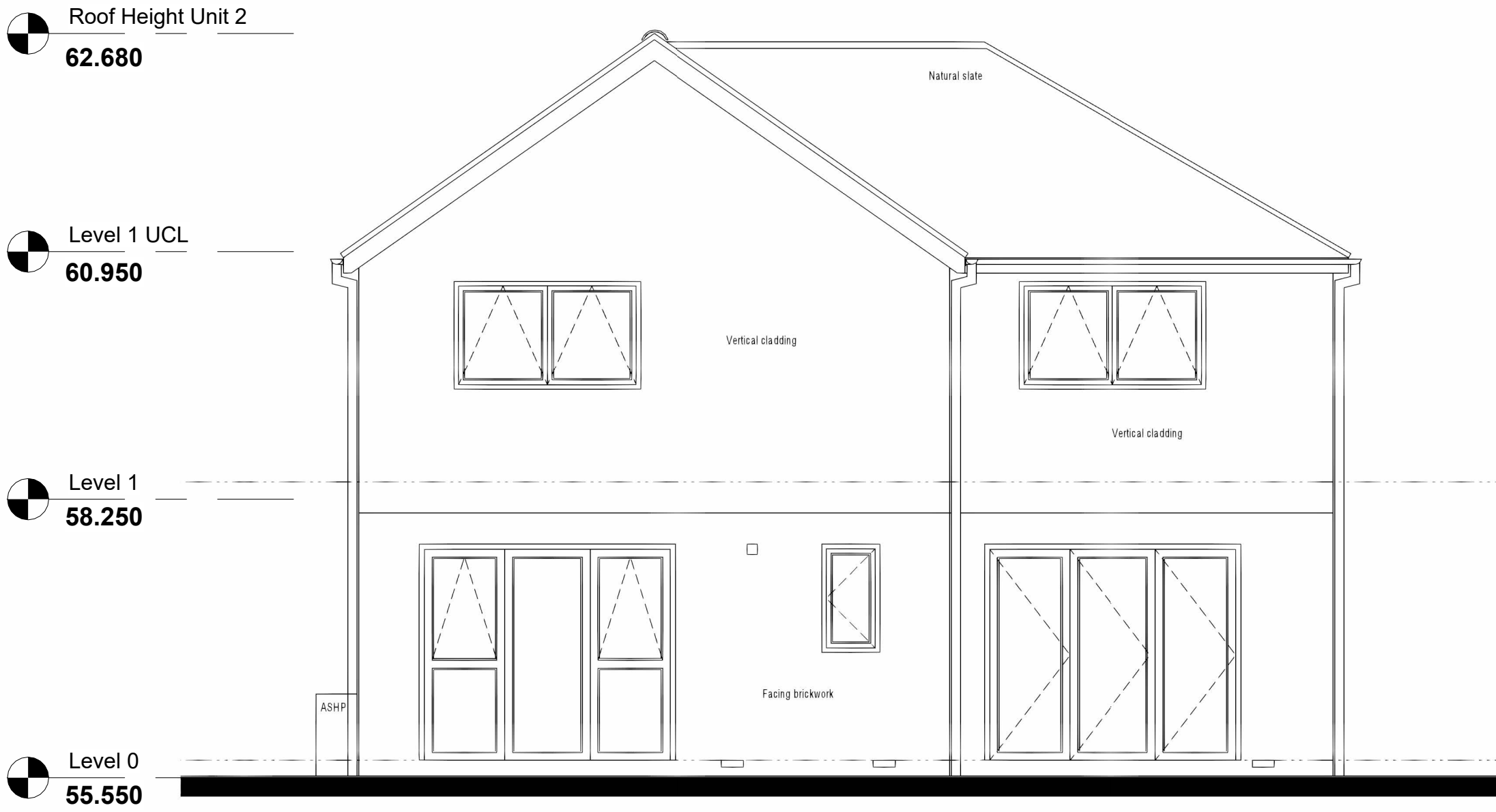
2 Unit 2 - Rear Elevation 1 : 50
