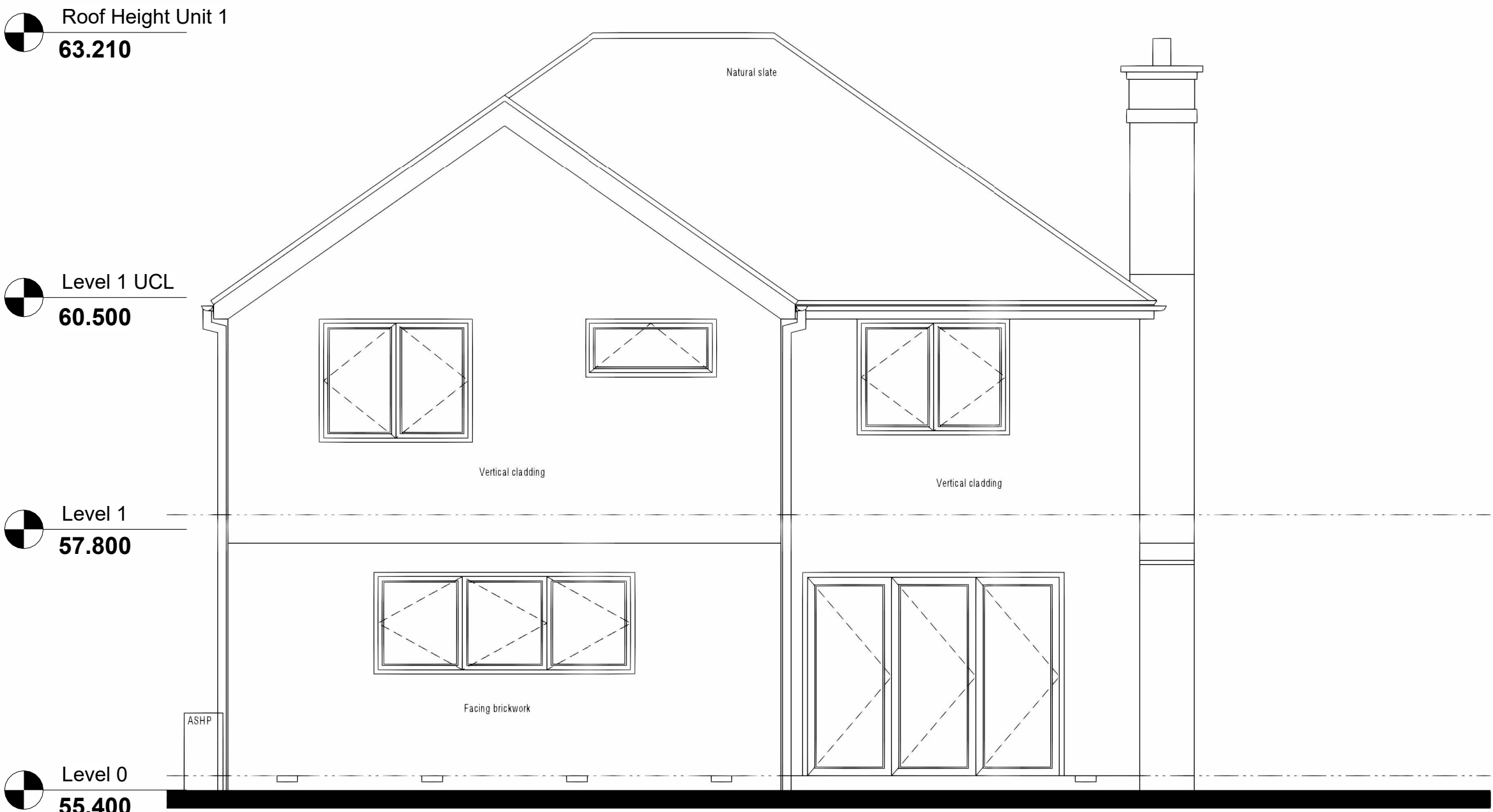
2 Unit 1 - Rear Elevation 1 : 50
