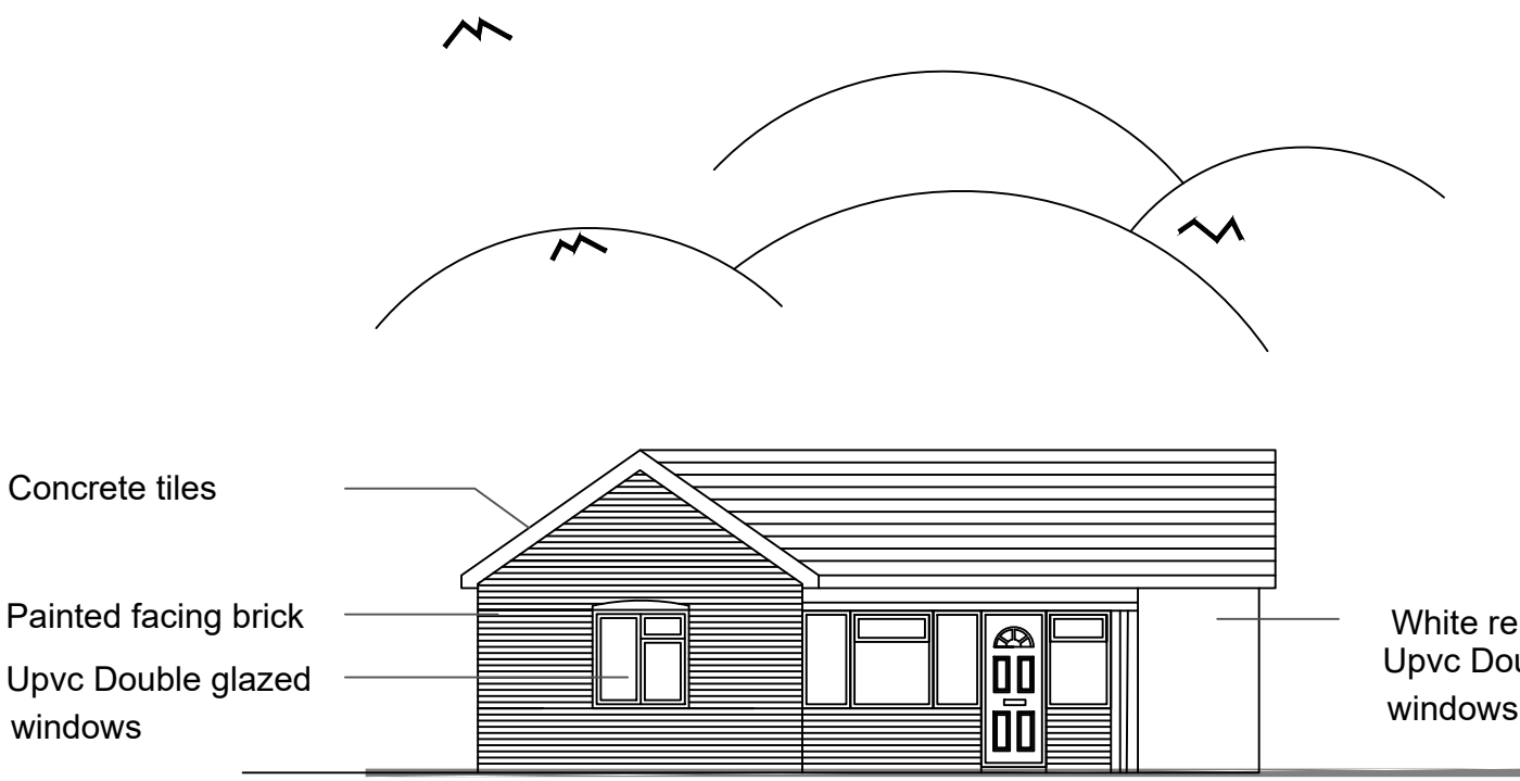
East Elevation Scale 1:100
