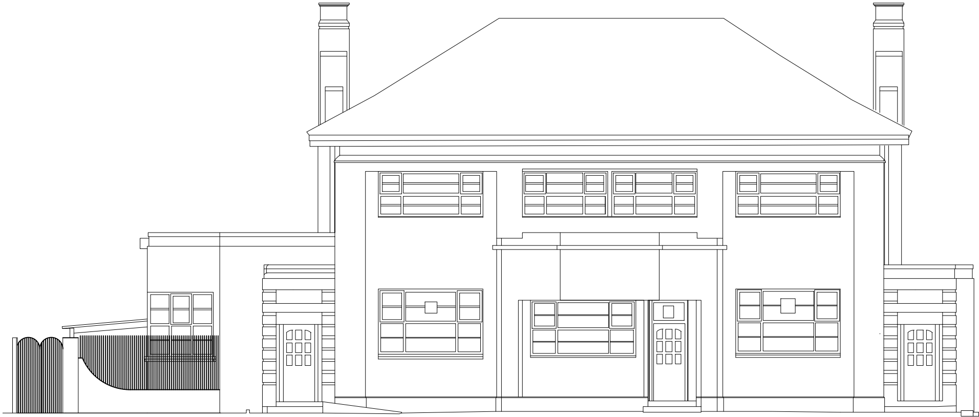
Existing front elevation scale 1:100
