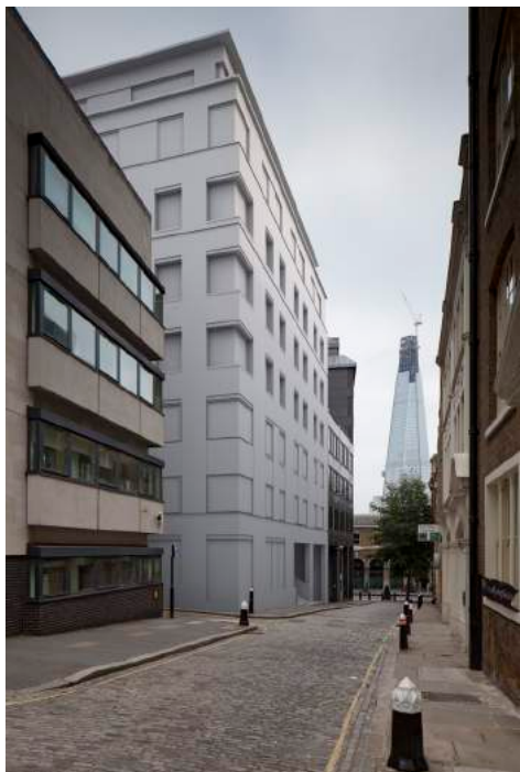
AVR2 (AVR Level 2) Explaining architectural form (in this case as a simply shaded render in a uniform opaque material)
