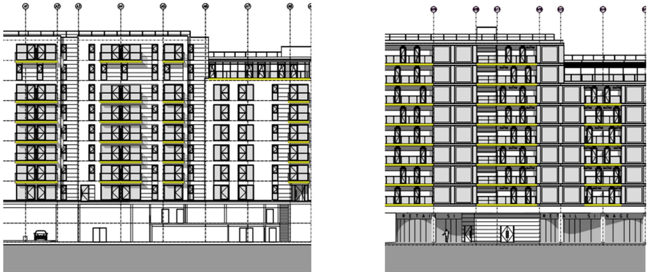
Fig. 8 – Typical East (Left Hand side) and West Elevations (Right Hand side) showing on the left-hand side the projecting balconies and on the right-hand side the recessed balconies
