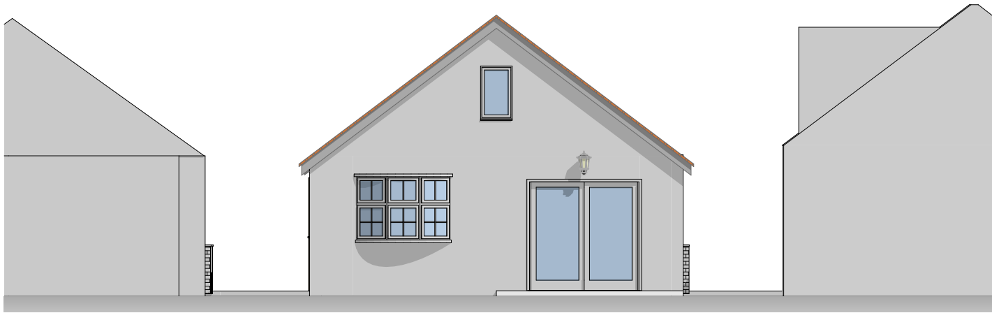
E-17 Existing Rear Elevation 1:100
