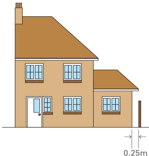
Single storey side extension
