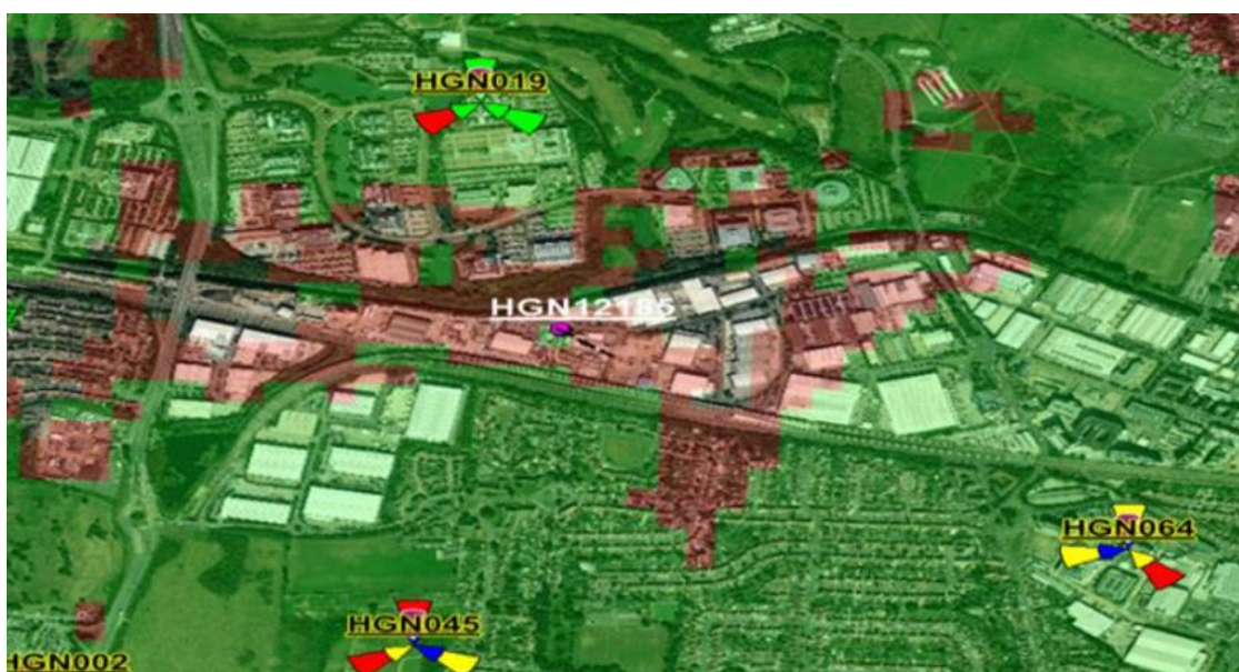
Figure 4: Coverage plot for the H3G 5G base station to be built at Shepiston Lane
