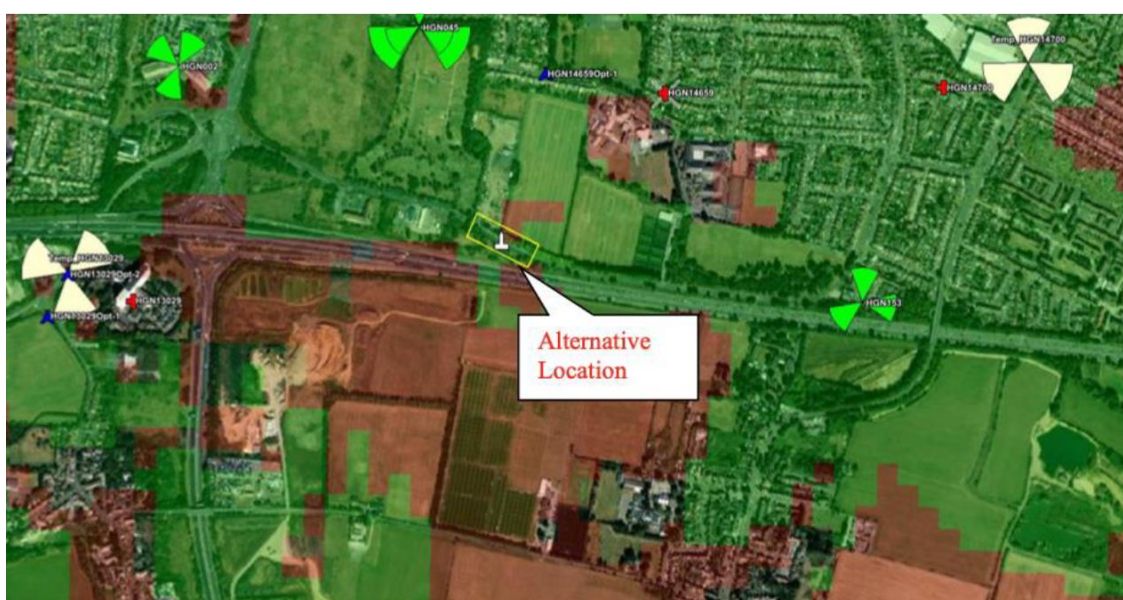
Figure 4: Coverage plot for the H3G 5G base station to be built at Shepiston Lane
