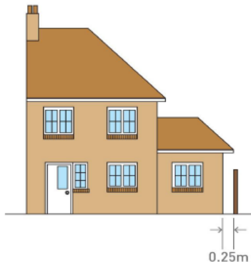
Single storey side extension
