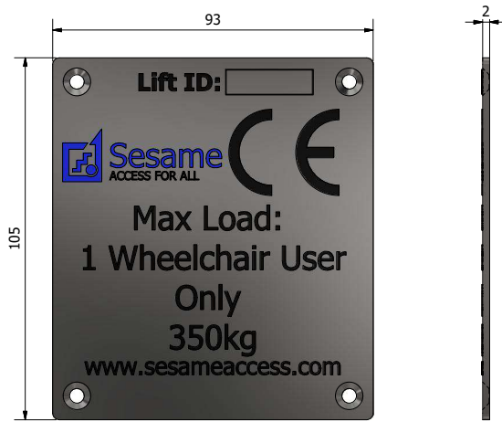
Safety Working Load Plate Located on Lift Button Station
