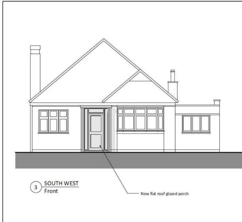
Figure 4: Excerpt from the proposed plans showing the proposed front elevation.
