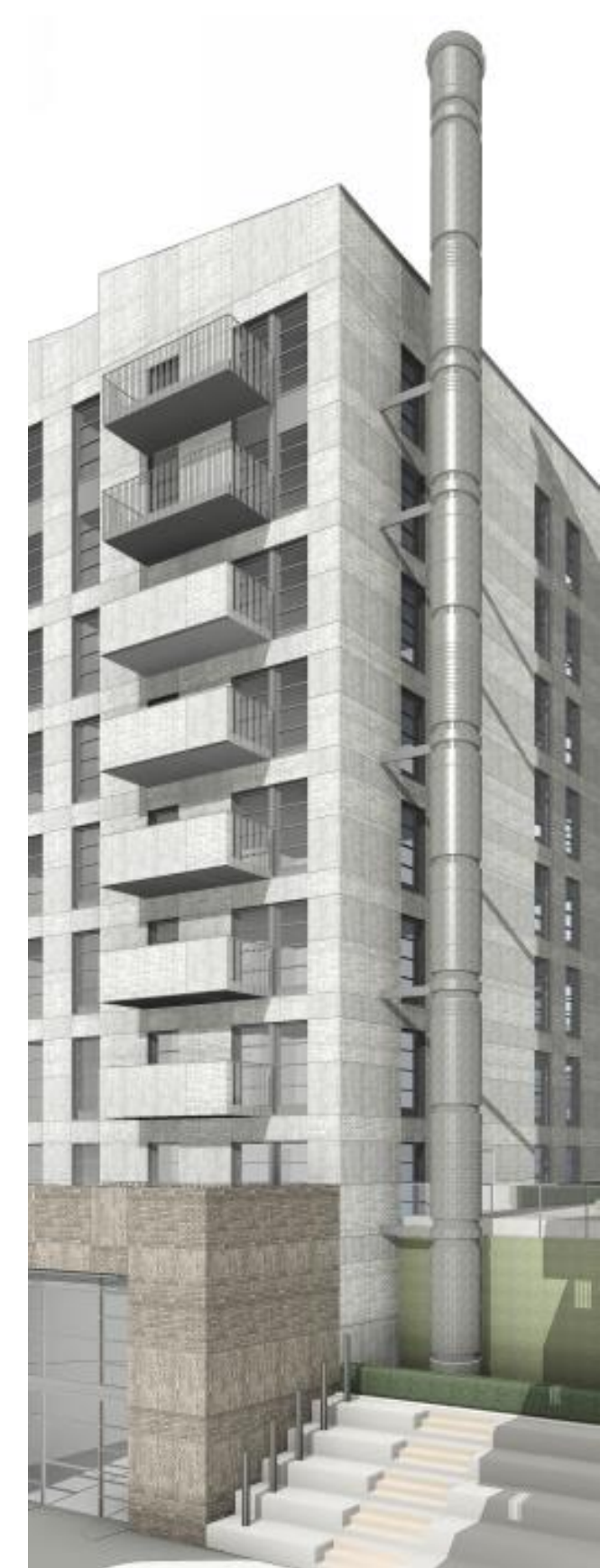
Figure 20 Flue Access Via Rope Access Monorail at top
