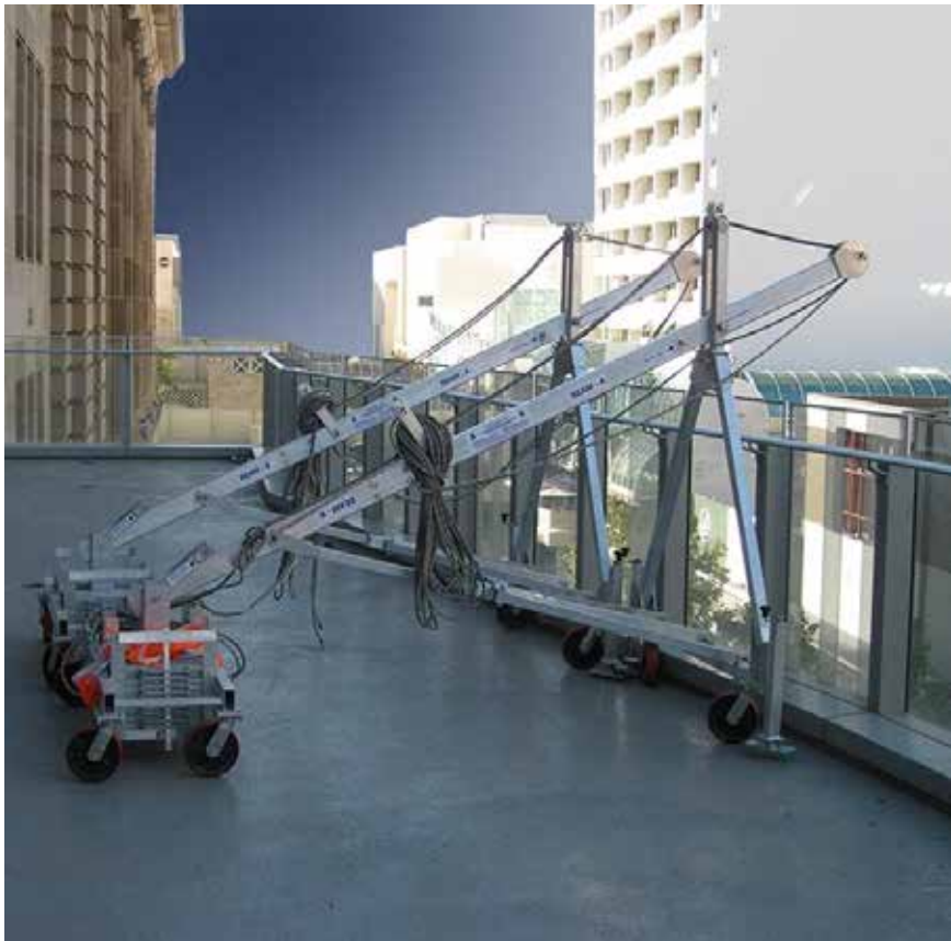
Figure 23 Temporary Counterweighted Davit (TCD)
