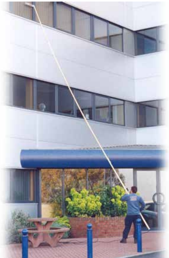
Figure 12- Deionised Water Fed pole up to 12m maximum
