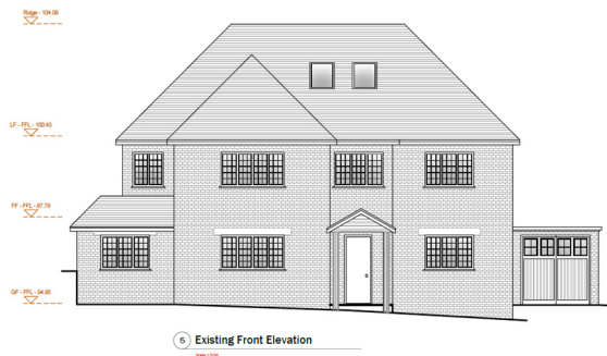
Existing Front Elevation
