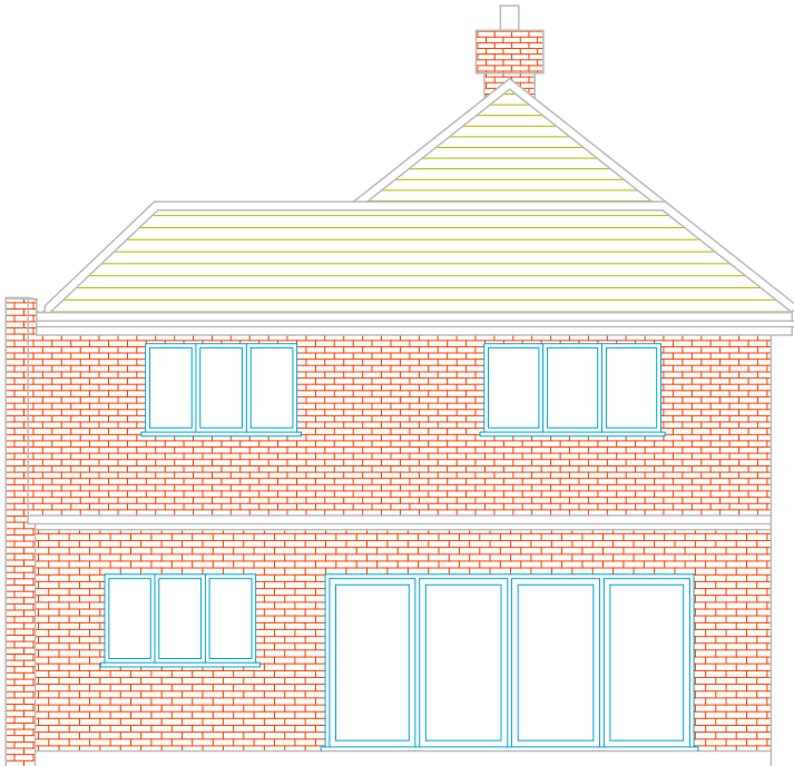
PROPOSED REAR ELEVATION
