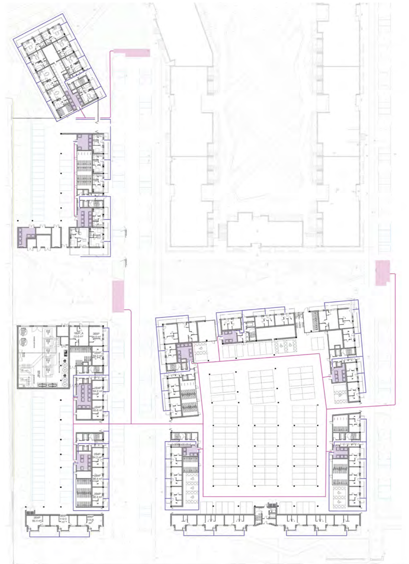
Fig. 2.8.10: Servicing Strategy - Block C, D and E layout showing the distribution of the bins storage
