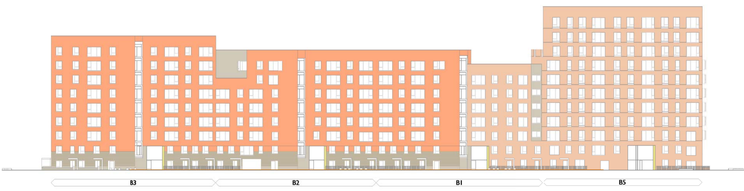
CANAL STREET ELEVATION - BLOCK B Brick Types 1: 500
