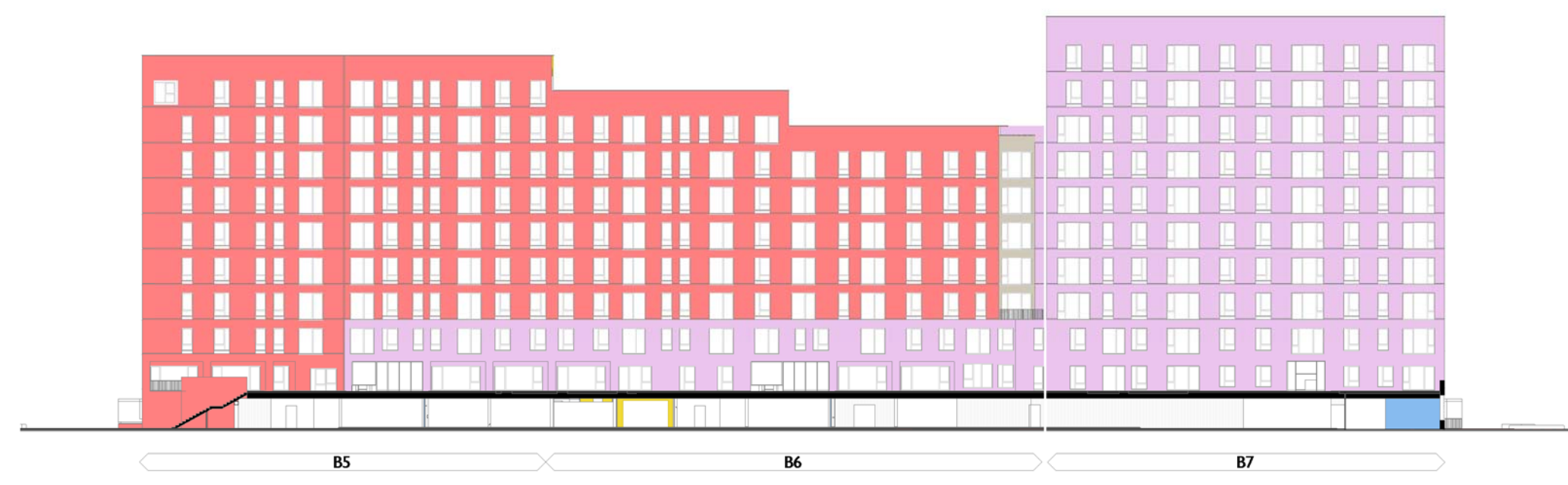
COURTYARD EAST ELEVATION - B Brick Types 1: 500
