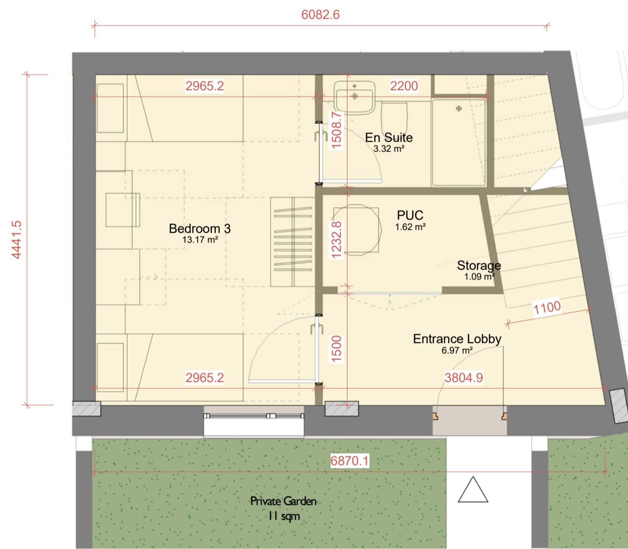
3 BED DUPLEX UNIT - GROUND FLOOR
