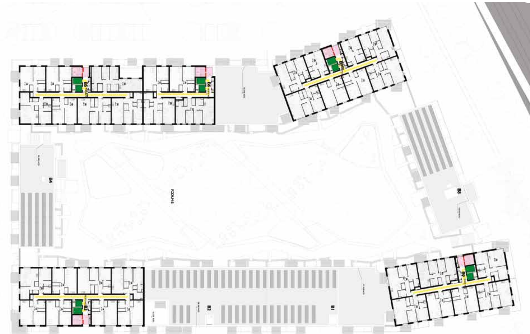
Fig. 5.2.5: Block B General Arrangement-Eighth floor
