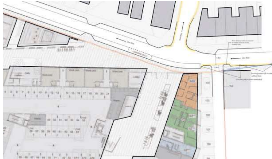
Fig 6.1 - Ground Floor Plan with loading bay for service vehicles.
